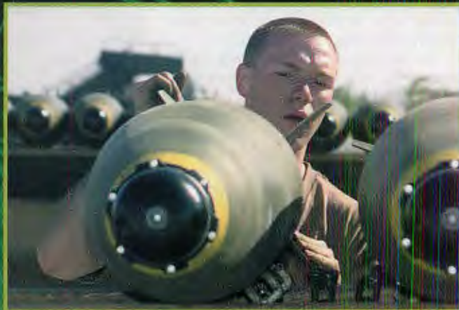
Weapons load crewmember, Airman Todd Sturz secures a bomb-lift strap to an MK82 general purpose bomb before uploading into a B-1 bomber from Dyess.
